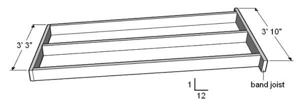
The top band joist will extend 3 ½" beyond the outside of the runners on either side (as seen below). The bottom runner will end flush with the outside of the runners.
