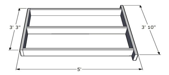
Each panel will be bolted to 4x4 treated posts and to each other, through the band joist, with 3/8" x 7" lag bolts.
