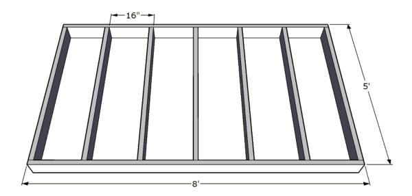
Each panel will be bolted to 4x4 treated posts and to each other, through the band joist, with 3/8" x 7" lag bolts.
